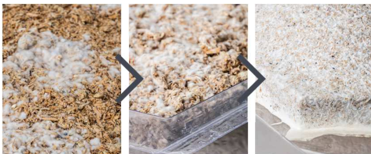
Mycelium acts as the main binding agent (glue) for the substrate, providing strength to the new bio-material
