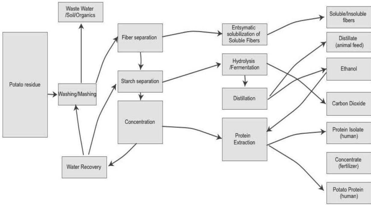
**Figure 18** Flow chart of value added products from potato residue feedstock [267].
