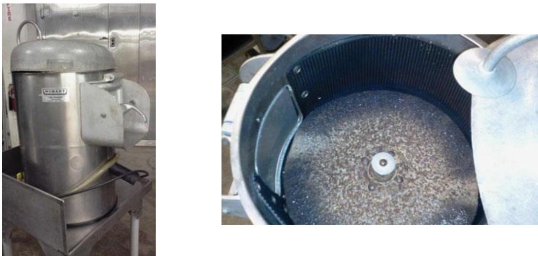
**Figure 7 (left)** Abrasion peeler for potatoes and sweet potatoes. **(right)** Rotating cylinder with an abrasive surface along the inner wall to remove the skins as the cylinder rotates.
