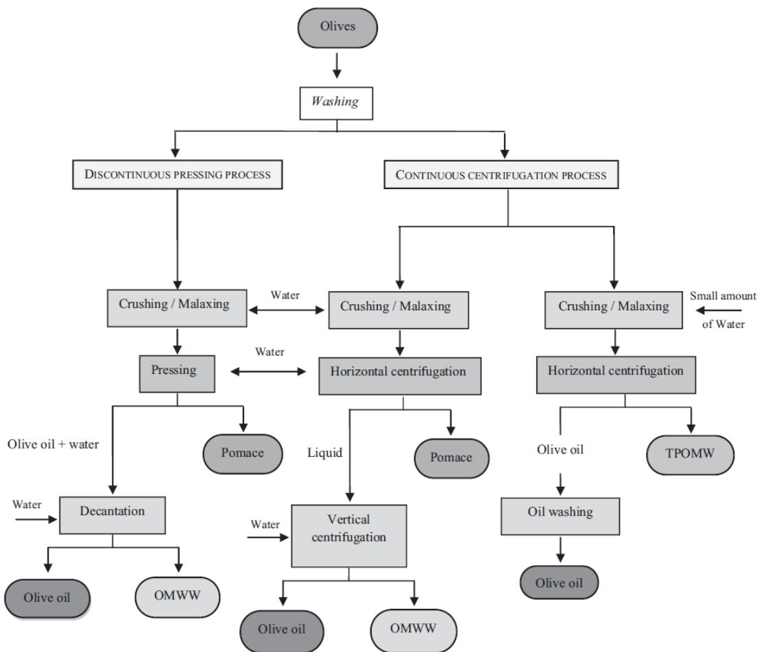
**Figure 17** Main processes for olive oil extraction [138].
